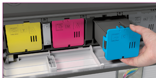
Toner cartridges automatically eject only when fully exhausted.
